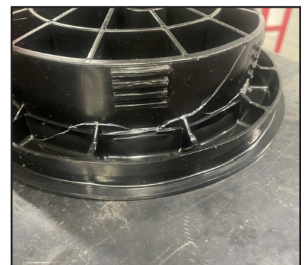
Cracks in support structure
